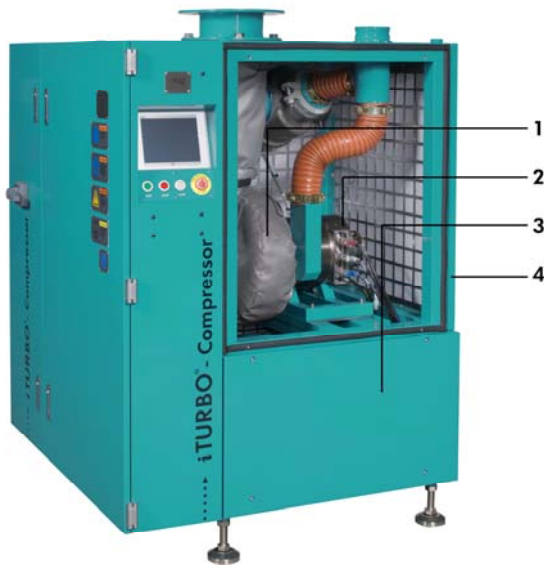
iTURBO® – Compressor (panels removed)
